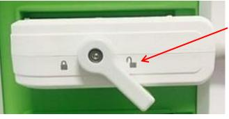
Transducer connector lock knob (in the unlocked position)
