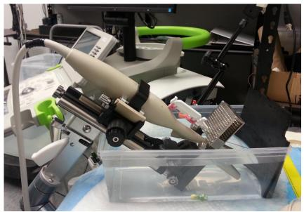
Figure 41: Transducer and Transperineal Stepper in Water Bath
